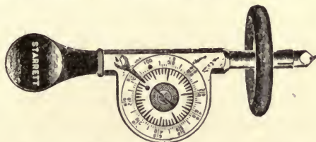
B. A Surface Speed Indicator
